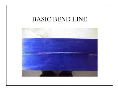
The basic layout is as follows. What you need to know includes, material thickness, degree of bend and bend radius
