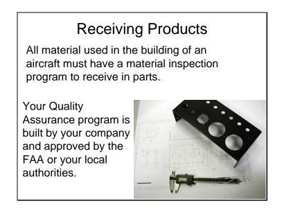
All material used in the building of an aircraft must have a material inspection program to receive in parts.
