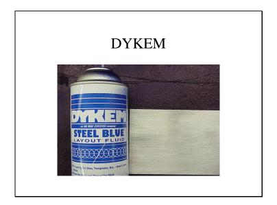
Dykem's Steel Blue Layout Fluid is a blue spray that is used to see scribe lines on the Master Tool.
