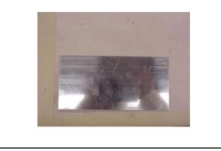
Aluminum is one of the most widely used metals in modern aircraft construction. It is vital to the aviation industry because of its high strengthto-weight ratio and its comparative ease of fabrication. The outstanding characteristic of aluminum is its lightweight. Aluminum melts at the comparatively low temperature of 1,250 degrees Fahrenheit.
