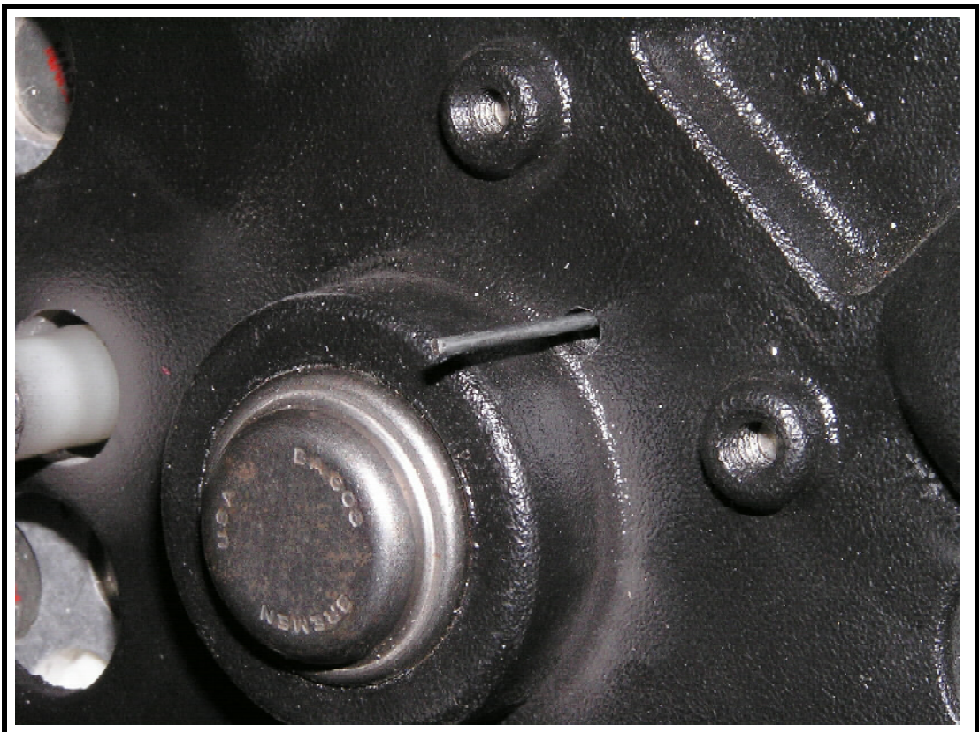
Brush Retaining Pin Installed to Hold Brushes In Place
