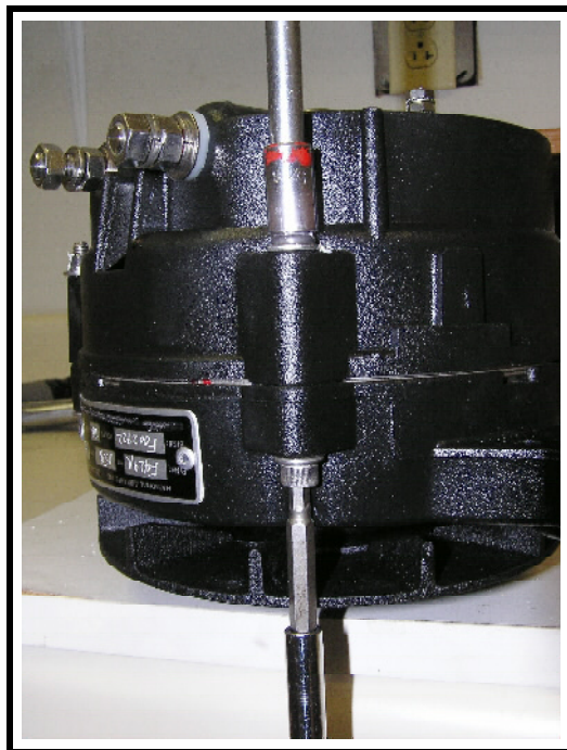
Thru Bolt removal on holding fixture. Thru bolt installation uses same procedure.
