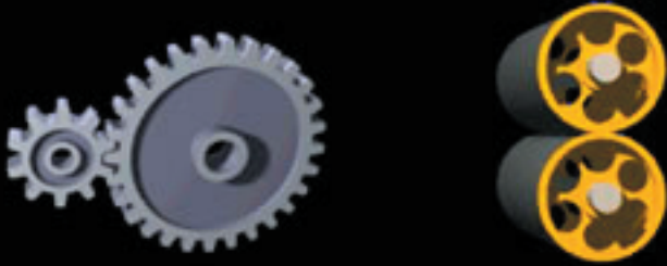
Common nip points on rotating parts
