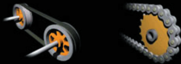
Nip points between rotating elements and parts with longitudinal motion
