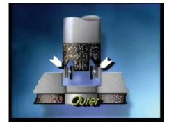
This bearing fits tight on the housing. Pressure should be applied to the top of the outer race.
