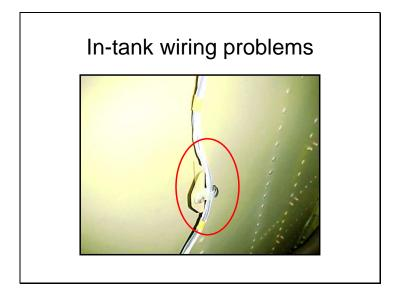
In this picture we see the wiring is rubbing against the bracket and wall of the tank
