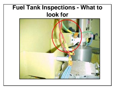
Fuel Quantity Indicating System and fuel pump in-tank wiring problems discussed herein
