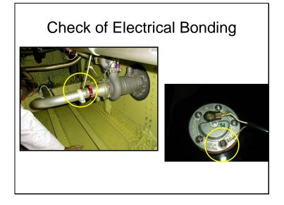
Check Electrical Bonding Straps or bonding points
