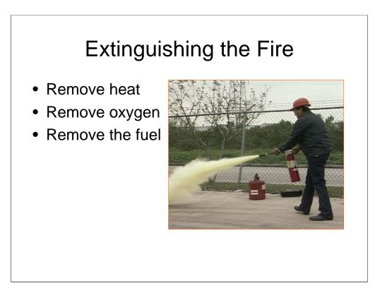
Fire extinguishers are designed to remove at least one of the three elements so that a fire will die out.
