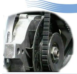
Alternator Basics The self rectifying alternator has the means to generate AC and rectify it back to DC.
