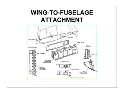
**The WING-TO-FUSELAGE ATTACHMENT** structure constitutes the center box structure and is designed to form the structural tank.
