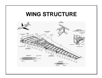
The structure of each wing is basically composed of aluminum alloy panels attached to two spars and twenty two ribs.
