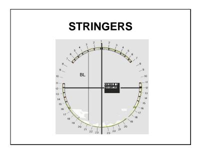
Stringers are placed like minutes on a clock about a 10 inch spacing Right hand stringers are R1 R2 R3 ex and left hand stringers are L1,L2L3L going clockwise. L
