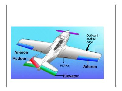
Listed are the basic flight control surfaces. larger aircraft flight control systems may include fly by wire systems. While smaller aircraft may use hydraulics or more simplified systems. The flight control surfaces listed here are the basics of a small aircraft.
