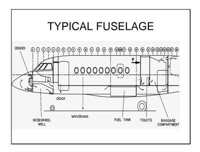
The typical fuselage has windows, floors, and doors to enter the cabin It also contains the seats, aircraft electrical systems, Hydraulic systems, flight control system, toilet, drinking water, storage cabinets and avionics systems.
