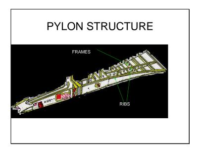
Pylon Structures are made of ribs and frames.
