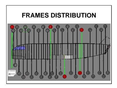
Frames are distributed forward going aft. the circles in the visualization identify the frames- example 7 frames aft of frame 0 is **frame 7**
