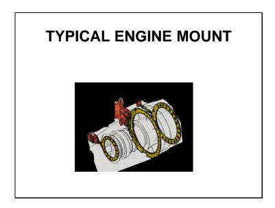
Engine mount structures. Because of their purpose and location engine mount structures are subject to extreme heat, vibration and torque. To withstand the demands imposed on them, these structures may be constructed from welded tubular.
