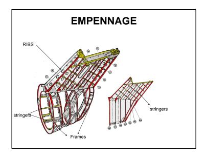
The empennage is made up of Frames stringers and Ribs This gives the tail section its strength.
